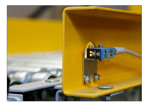
Figure 1. Many discrete sensors are available with IO-Link, so they can provide advanced data and connectivity, going far beyond basic on/off signals, with simplified field installation.
