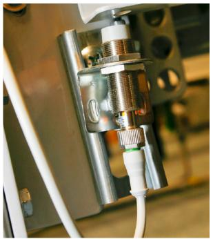
Figure 2. Proximity sensors using capacitive, magnetic, or inductive technologies are a compact way of detecting various targets.
