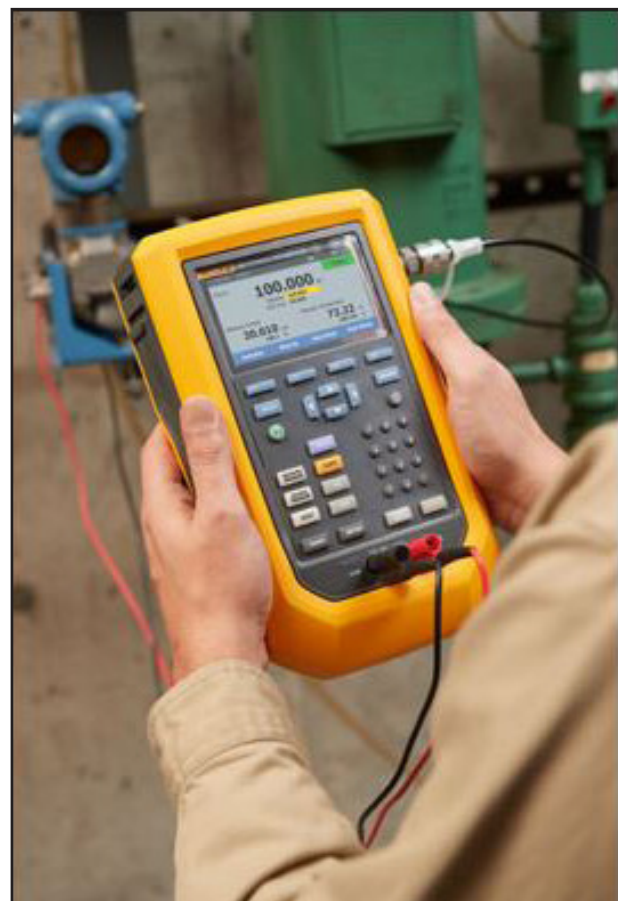
Figure 1. Fluke 729 provides a big productivity boost for pressure calibration.
