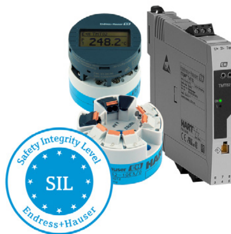
Figure 3. Some temperature transmitters have a two-channel function that can detect drift between sensor 1 and sensor 2, a broken sensor, and corrosion on the sensors, as well as provide automatic sensor backup if one sensor fails.
