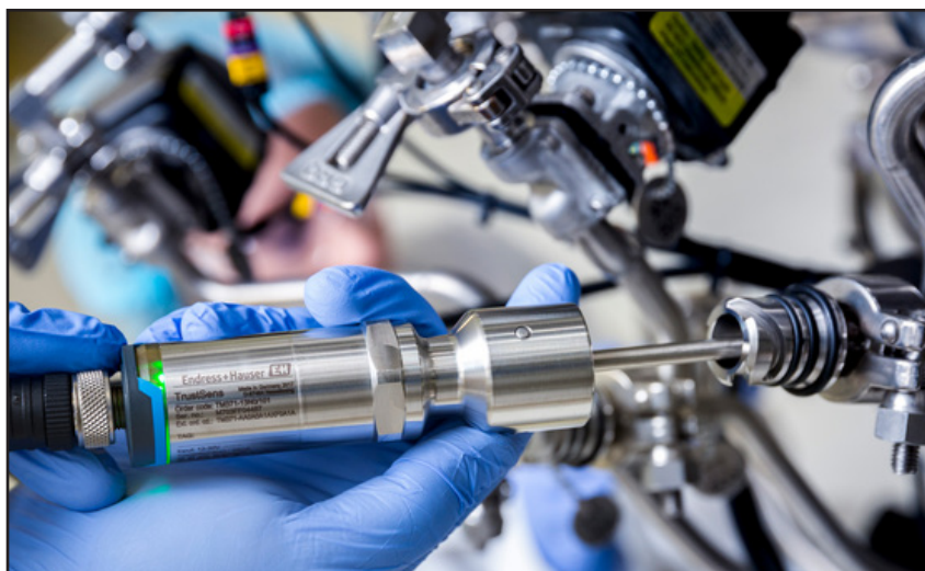
Figure 5. A quick disconnect feature can reduce calibration and downtime while reducing risk by eliminating the need to remove leads from the transmitter.
