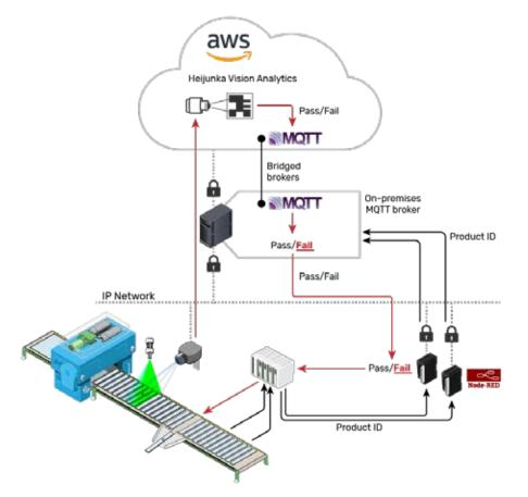
A hybrid architecture using two groov RIO modules on each production line to allow cloud-hosted analytics to securely control action in the physical process at the edge of the network.
