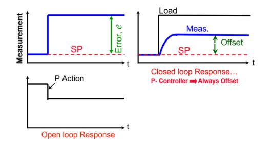
Figure 2. Proportional only controller response to a change in load.
