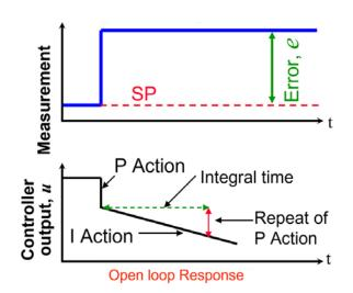
Using the integral of the error to eliminate offset
