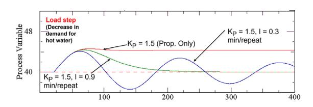
Using the integral of the error to eliminate offset
