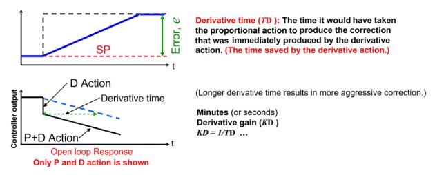
Figure 10. Proportional plus derivative controller response to a load change in an open loop.
