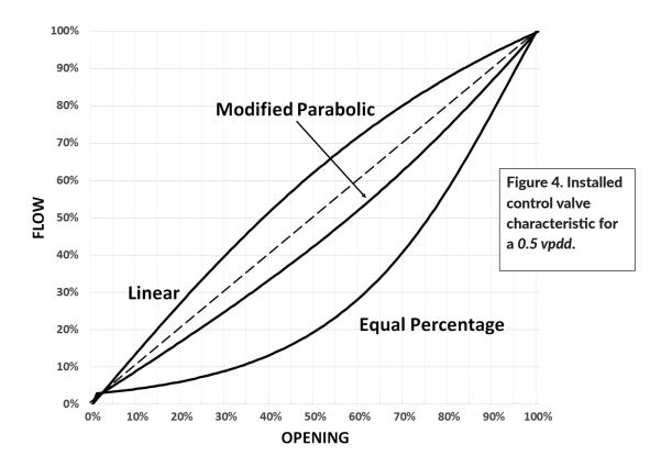
pressure drop decay (*vpdd*), then the "installed control valve characteristic" will be different, changing the proportion from controller signal output to the control valve flow.
