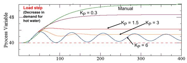
Figure 4. Process variable response to a load step change with varying proportional gain settings.
