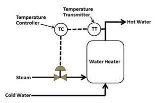
Figure 3. A simple control loop.
